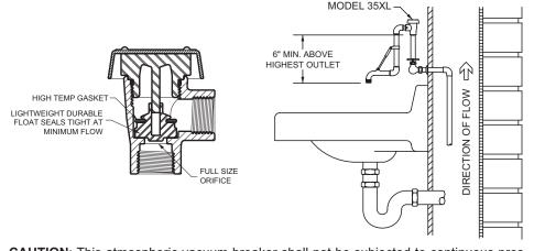
**CAUTION**: This atmospheric vacuum breaker shall not be subjected to continuous pressure for more than twelve (12) hours. The device shall be installed in accordance with the requirements of the local plumbing code. The device shall not be installed where the venting of water from the device during its normal functioning causes damage. The device shall be installed downstream of the last valve, therefore never place a shut off or check valve downstream of AVB's.
