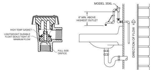
**CAUTION**: This atmospheric vacuum breaker shall not be subjected to continuous pressure for more than twelve (12) hours. The device shall be installed in accordance with the requirements of the local plumbing code. The device shall not be installed where the venting of water from the device during its normal functioning causes damage. The device shall be installed downstream of the last valve, therefore never place a shut off or check valve downstream of AVB's.
