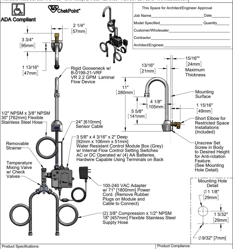
Chrome Plated Brass Electronic Faucet: Wall Mount Rigid Gooseneck w/ VR 2.2 GPM Laminar Flow Device, AC/DC Control Module with Internal Flow Control Setting Switches, Temperature Control Mixing Valve w/ Check Valves and 18" Flexible Stainless Steel Supply Hoses
