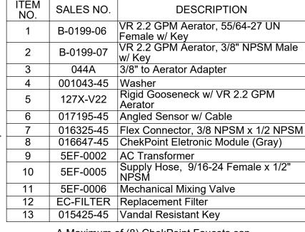
A Maximum of (8) ChekPoint Faucets can be Hardwire Connected and Powered by EC-HARDWIRE ChekPoint Hardwire AĆ Transformer. (Sold Separately)
