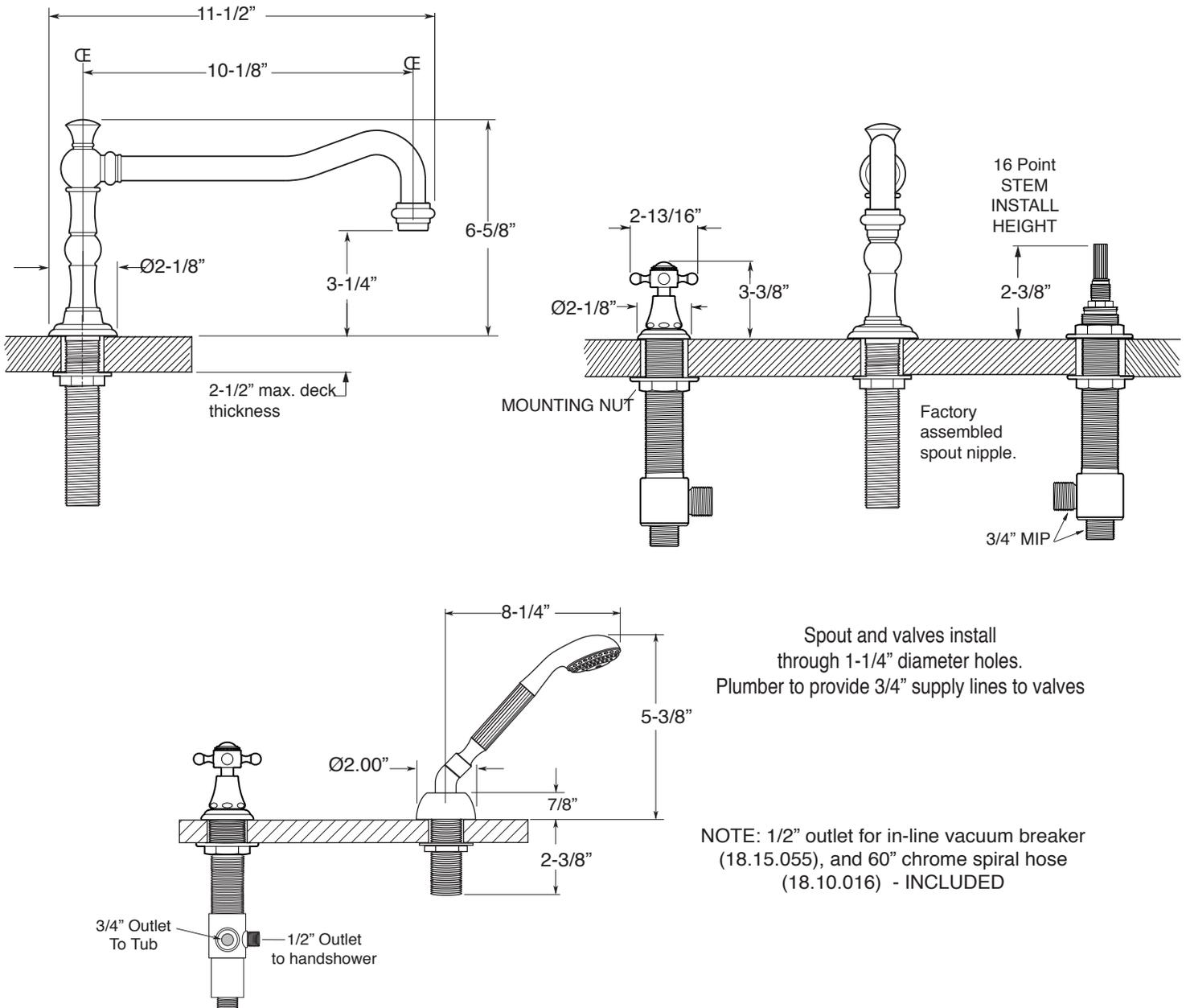
Spout and valves install through 1-1/4" diameter holes.
