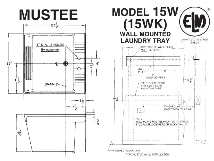
1. Secure **Wall Plate** to wall using both 5/16" x 2" **Lag Screws**. Locate mounting holes 1-1/2" below desired tray height as measured from top edge of rim.
