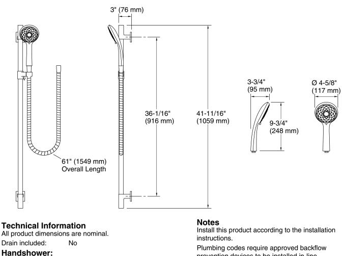
Rated maximum 2.5 gal/min (9.5 l/min) flow: Pressure: 45 psi (3.1 bar) Plumbing codes require approved backflow prevention devices to be installed in-line to handshowers. Please consult with local plumbing officials.
